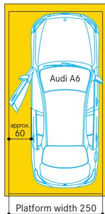
Depending on the vehicle model and the parking position of the vehicle on the platform, the space for opening the door varies. We recommend platform widths of 250 cm.
